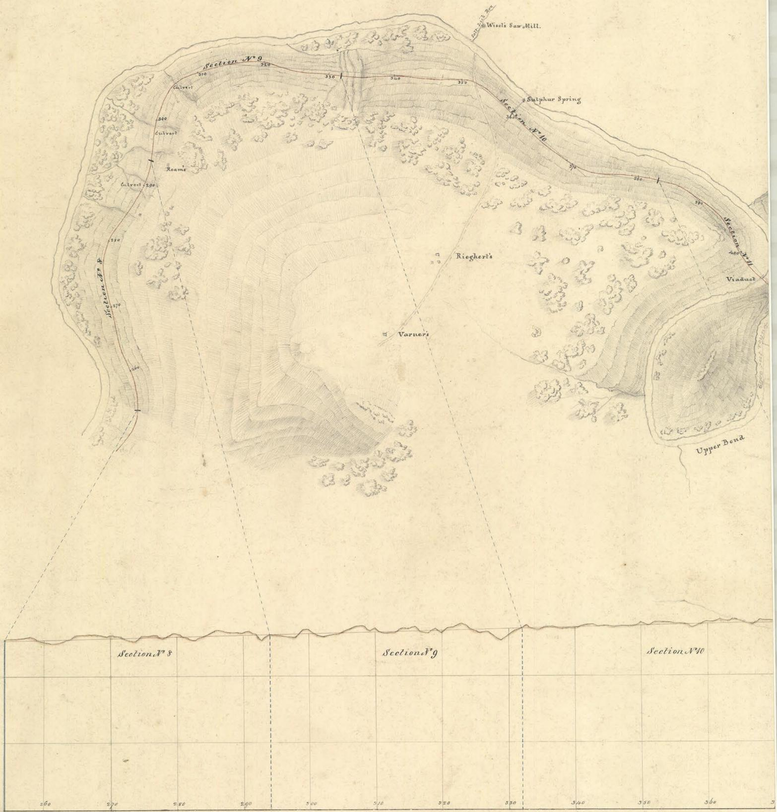
Length 4000 feet. The greatest portion of the work will be common excavation. There will, however, be some Embankment and some Solid Rock. The materials to form the Embankment will be taken from the upper side of the road. Six drains to be built by Contractor, grubbing throughout section.
