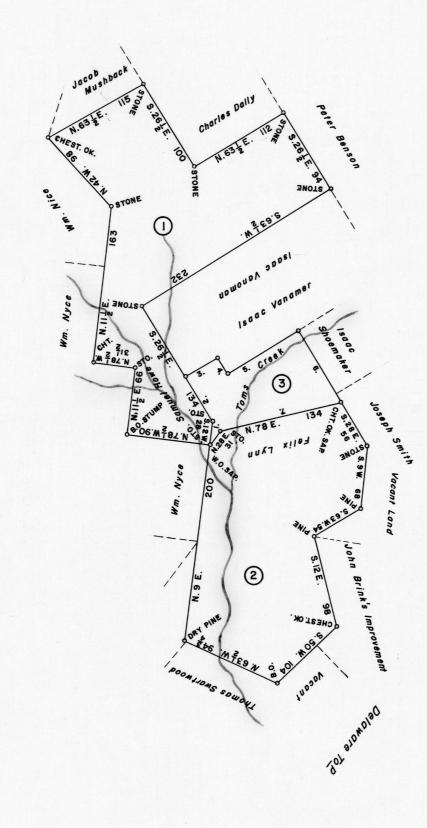
A CONNECTED DRAFT: of three (3) tracts of land which, when surveyed, were situate as follows: one (1) on Swartzwoods Mill Creek, Northampton County; and two (2) in Lehman Township, Pike County. The draft has been constructed from and compared with the original records on file in the Bureau of Land Records of the Department of Internal Affairs, Commonwealth of Pennsylvania, under the direction of Anthony G. Reese, Director.
